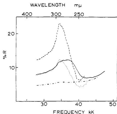
**Figure 1.** Polarized single-crystal reflection spectra of 6-azauracil obtained with light whose electric vector vibrates parallel to *a* (---), *b* (- - -), *c* (—), and a direction in the *ab* plane 60° from the *a* axis (····). These spectra were measured on the (010), (100), and (120) faces, and the *c*-axis curve is that obtained on all three of these faces. The (····) curve is referred to in the text as the *ab* spectrum.
